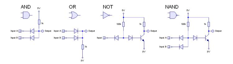
Logic Functions With Diodes And Transistors
